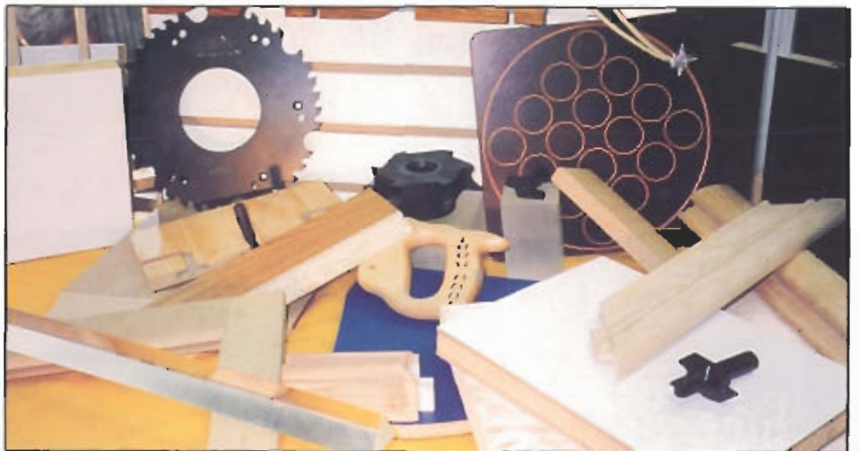
Figure 4 Diamond tipped tools are used to cut a variety of wood and plastic products.
